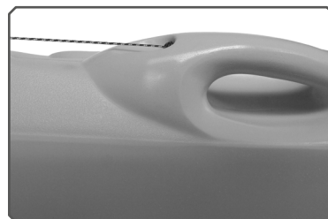
The Horizon has indents at the back of both rear handles. These entry points allow the lines to run through the inside of the rear handles rather than straight down into the boat.
